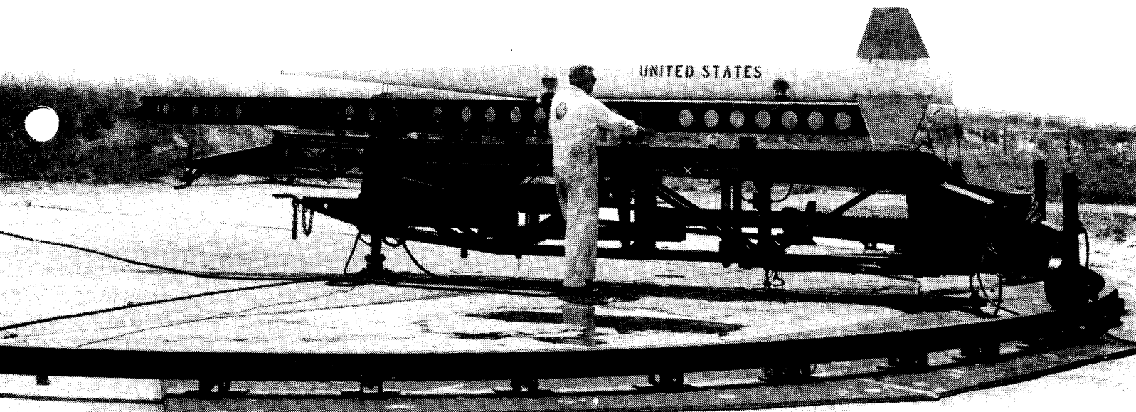
Nike Smoke test round (above) is prepared for launching from the Cape Kennedy sounding rocket site. Note the azimuth adjustment employing a semi-circular track system. (NASA Photo L-65-4760)
