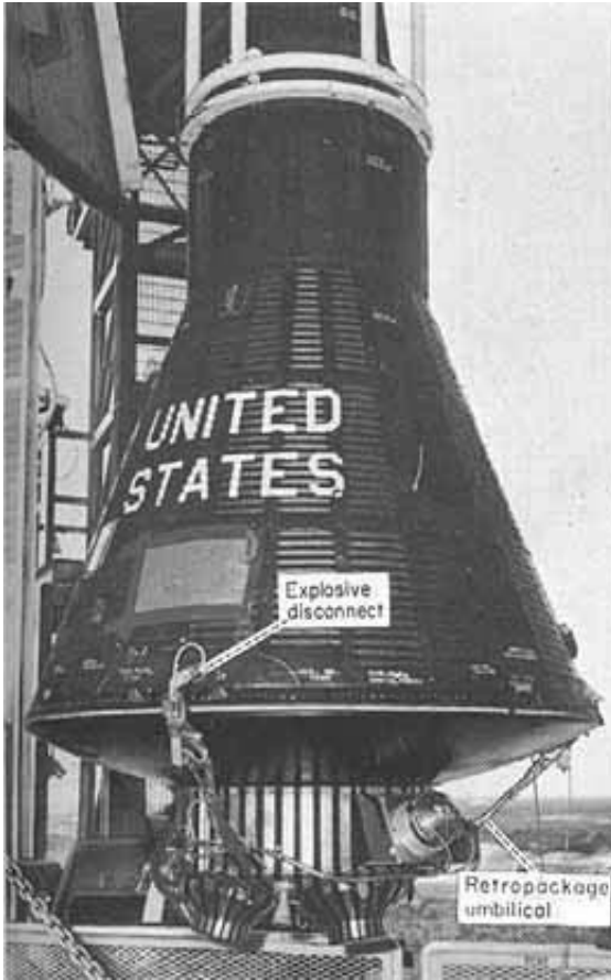
Figure 17 MA-9 Being hoisted to top of the Atlas
