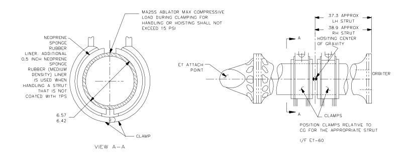
FIGURE 3.4-21.1 ET-60 ET/ORB FWD BIPOD STRUT HANDLING AND HOISTING I/F DETAIL
