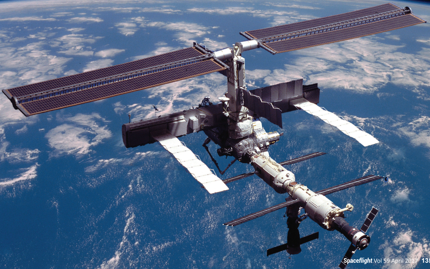
The ISS configuration with Truss segments S0, S1 and P1 installed during STS-113 in November 2002.
