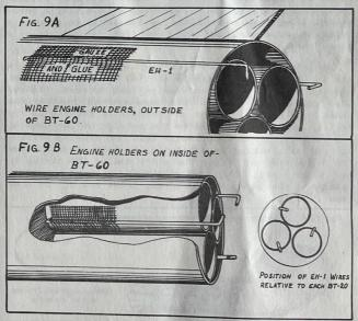
In the second system the engines are first glued or taped together, and then inserted into the rocket body. It is usually easier to obtain and maintain correct alignment by gluing the engines together than by taping them together. Enough tape is then wrapped around the outside of this group of engines to give a very tight
