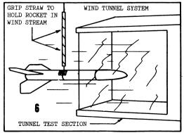
string. Apply a small piece of tape to hold the string in place. If the rocket's center of gravity (balance point) falls in the fin area, it may be balanced by hooking the string diagonally around the fins and body tube as shown in Fig. 5. A common straight pin may be necessary at the forward edge of one of the fins to hold the string in place. This string mounting system provides a very effective low friction pivot about which the rocket can rotate freely.
