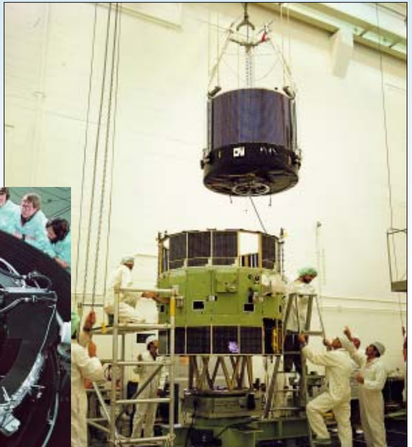
Mating ESA's ISEE-2 (top) with NASA's ISEE-1 at Cape Canaveral in preparation for launch.
