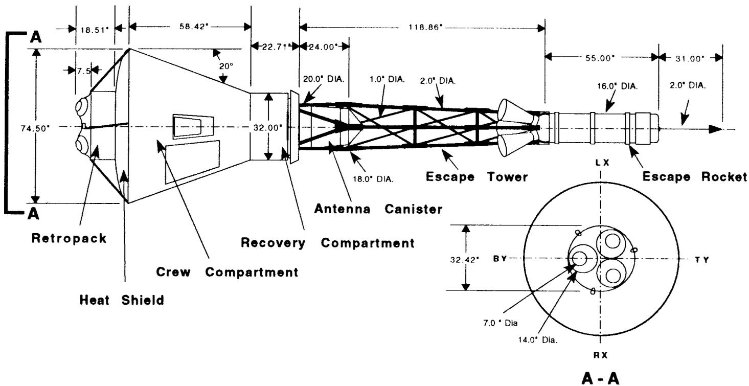
Figure 1. Mercury Spacecraft Basic Dimensions
