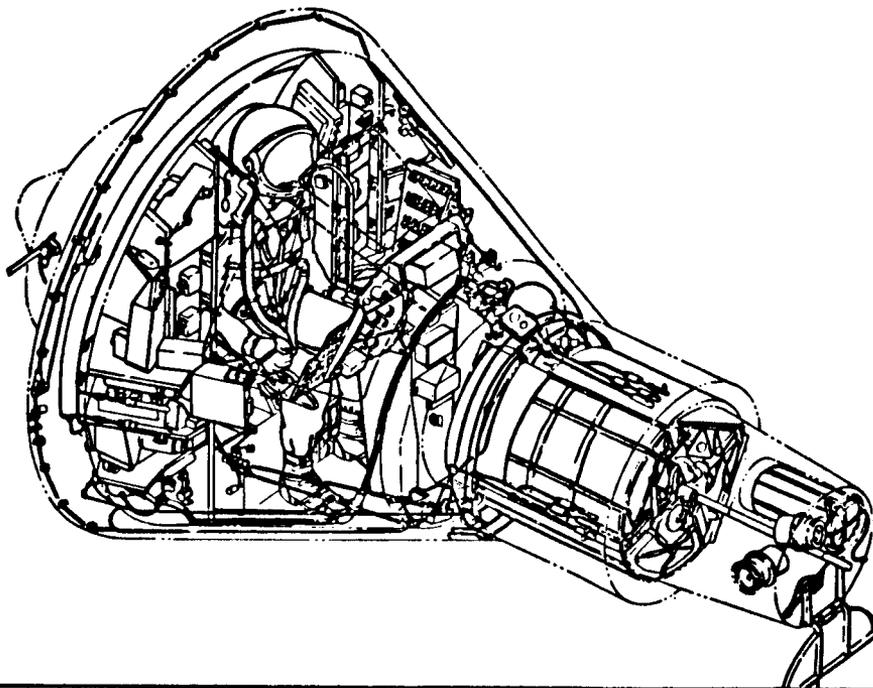
Figure 8. General Arrangement of Mercury Spacecraft
