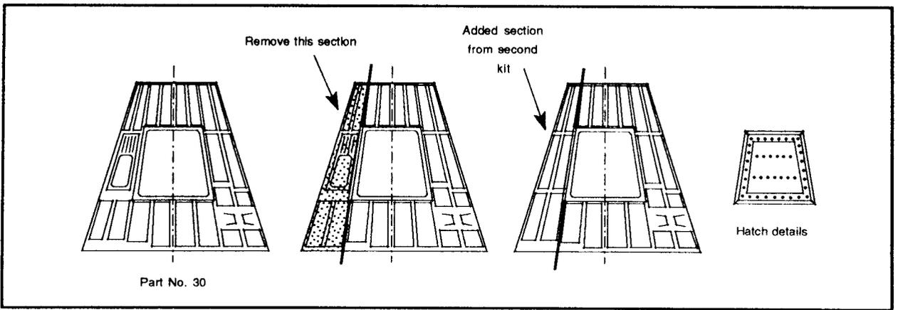
Figure 3. Part No. 30 revisions for spacecraft No. 7 details
