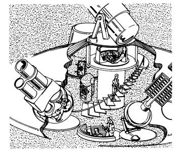
The Main Control Center of Pilgrim I contains all command, communications, control, and scientific experiment functions of Pilgrim I. Mounted on the MCC are the various antennas for communications, telemetry, and navigation. Several types of optical and radio telescopes will also be mounted for the MPEP phase of the Pilgrim I mission.
