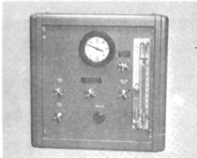
Figure 3-14. ALSD Pressurization Unit
