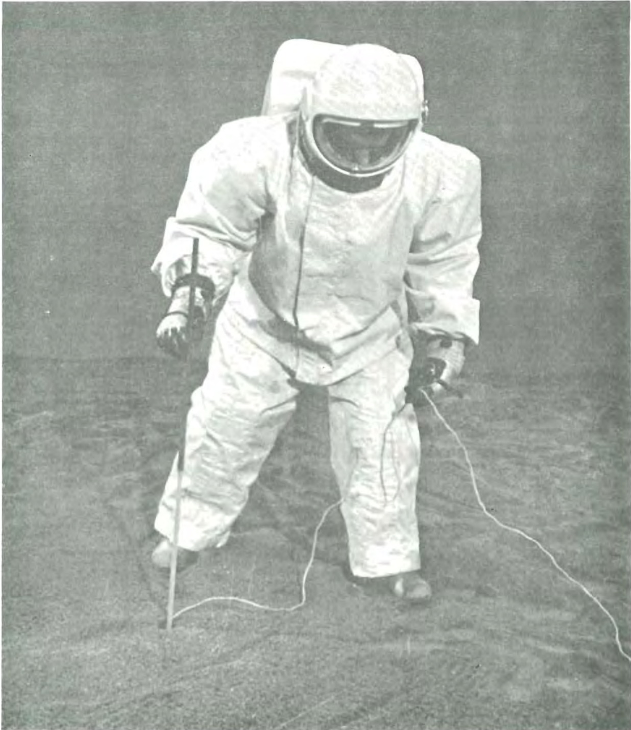
Figure 4-10. HFE Probe Emplacement
