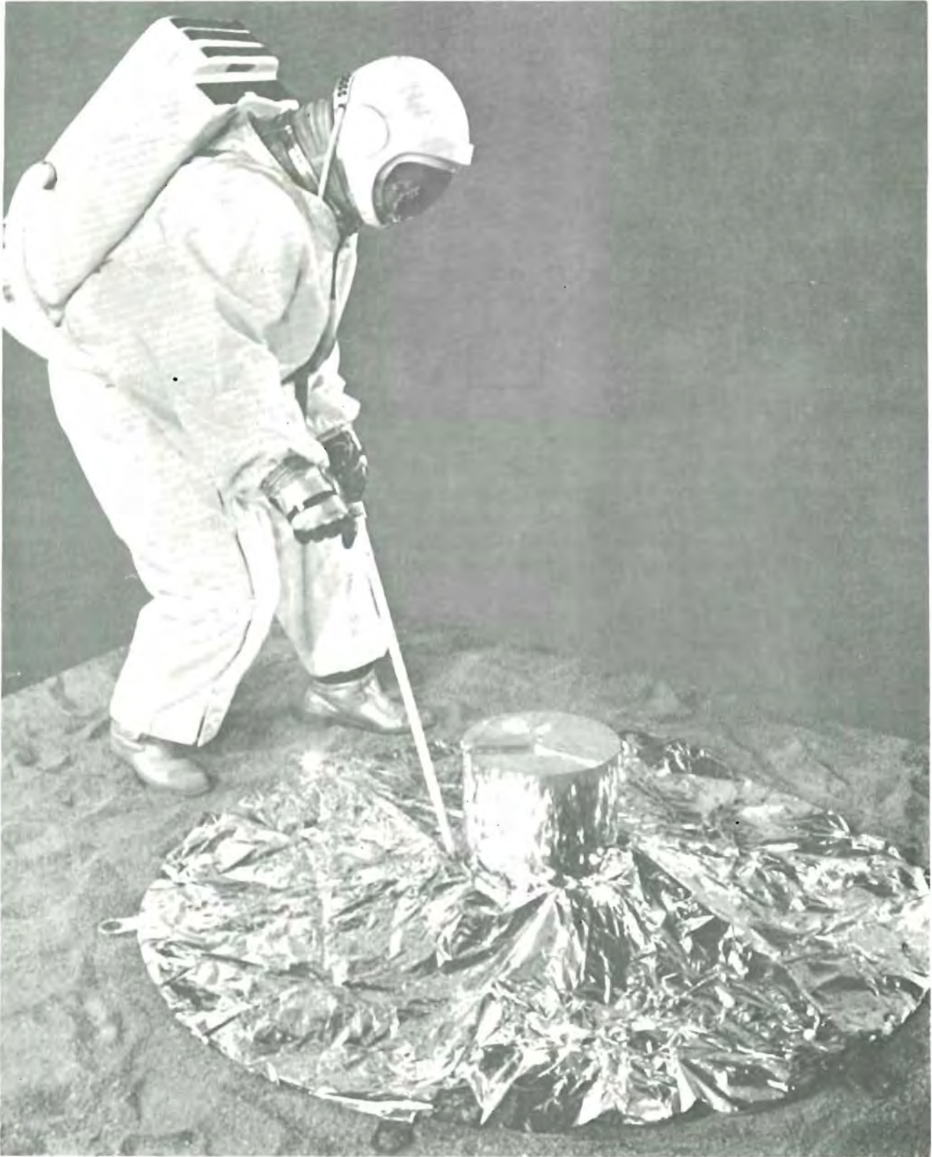
Figure 4-5. PSE Shroud Deployment and Experiment Leveling
