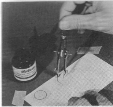
25. Mechanical drawing instruments are valuable for drawing perfect lines. Properly thinned Testors Pla or WATER-PROOF black drawing ink may be used.
