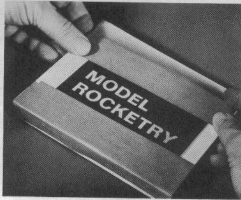
8. Water soluble gummed tape is good for masking the open area surrounding the stencil. Ordinary masking tape may be used if you don't plan to make more than a hundred copies.
