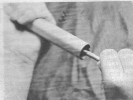
Figure 6. Holding the Peeler in the right hand (use a pliers to hold the flat end if it starts to slip), roll the tube using the left hand. Move the hand up the tube as it is peeled so that it is just ahead of the part that has just been peeled. This helps to reduce the chances of damaging the tube, but see the instructions for super peeling. If the Peeler comes loose, stretch the spiral out to the end of the tube, push the Peeler down the center of the spiral and reattach. Start rolling again.
