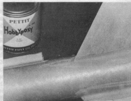
Step 11. Glue on the fins. When all the glue has dried, fillet the fin and launch lug joints.
