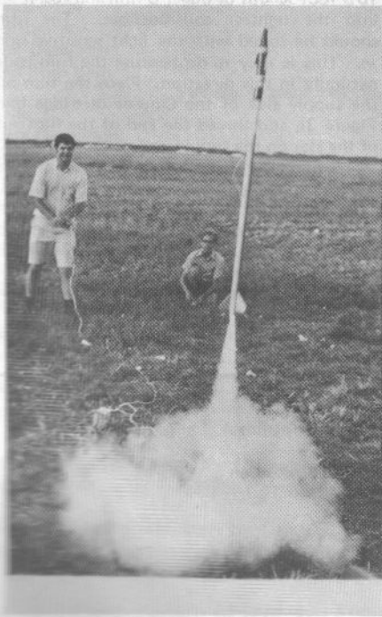
An F100 powered Cineroc carrier will provide an impressive high-altitude flight. The one shown above was the first launch of a Cineroc in conjunction with a Foucault in an attempt to obtain sound movies from the flight.
