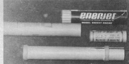
Step 14. The completed D engine adaptor and some engines the Giant Pipsqueak can be flown with.
