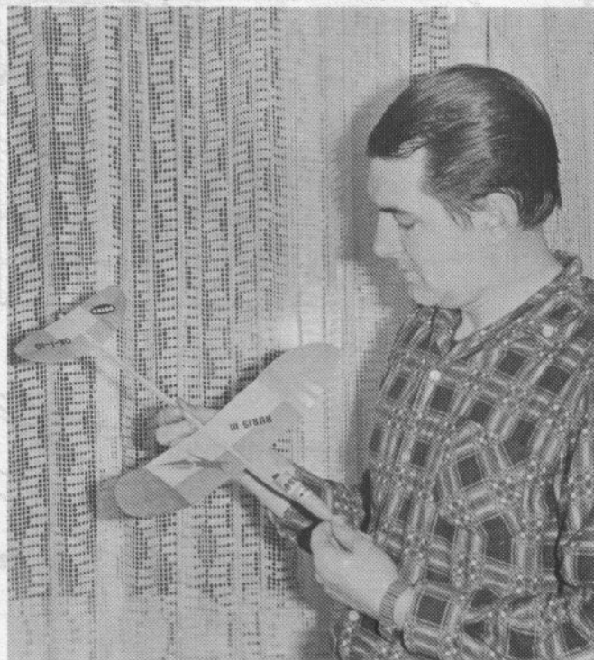
Jaroslav Divis of Prague, Czechoslovakia inspects his RUBIS III boost/glider. The glider uses an unusual technique of mounting the wing into cut sections of the boom to decrease weight. The original was scratchbuilt, including the tube, but standard parts can be substituted.
