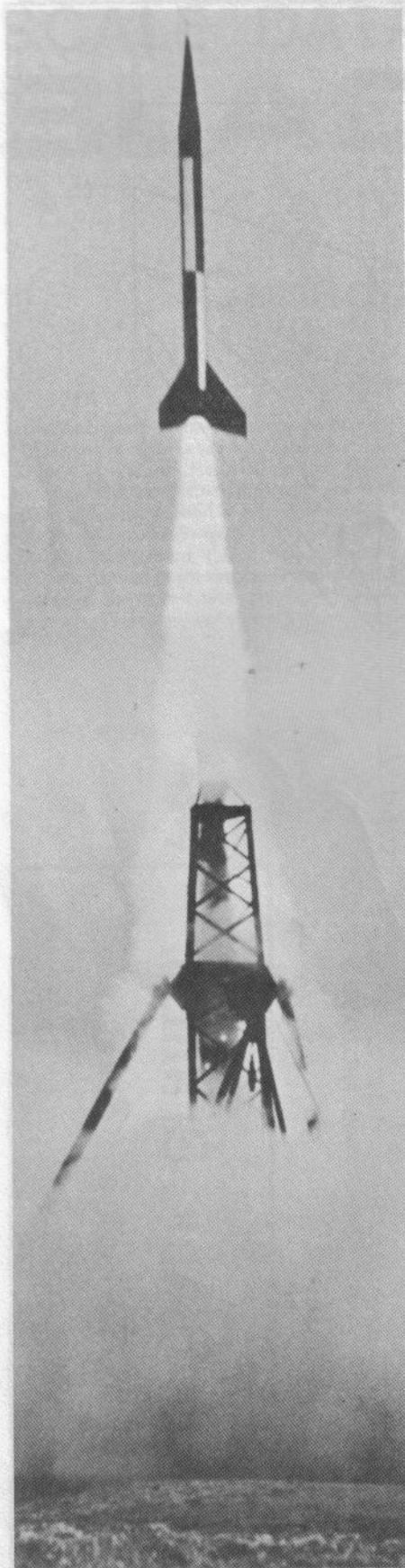
Liftoff from the Canadian Fort Churchill launch site of a test flight of the Black Brant II. Note the different roll pattern from the Wallops flown rocket. (CARDE photo No. 18722.)
