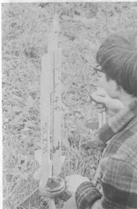
Dave Klouser's Hawk R/G entry -- Son of Groundhog -- was a C-powered swing-wing about the same size as Jon Robbins' A-powered Groundhog (see September '71 MRm for plans). The model boosted straight up, and turned in a 90 second duration for a full one minute lead over the second place entry.
