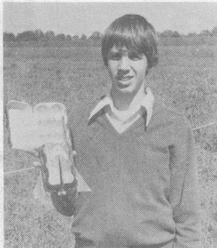
Roger Powell's unique sport egglofter was made from the packing box in which a dozen eggs are sold. The box was flight converted and flown with two eggs in place at the top.
