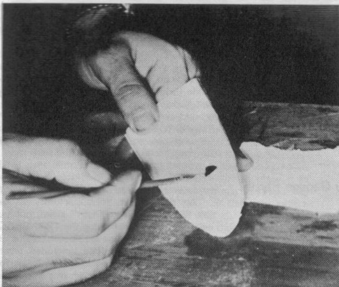
4. Brush a thin coat of epoxy over both sides of the wing. Make sure to cover the entire wing.
