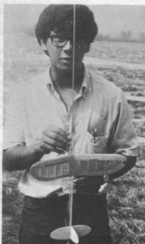
The Medina Team built-up wing R/G used a moving engine pod to shift the CG into position for a 19 second duration.
