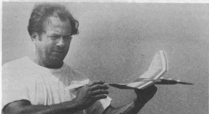
Bill Fileccia used the free-flight technique of downthrust (note pod angle) and side thrust to build this "no moving parts R/G" which turned in 98 seconds.
