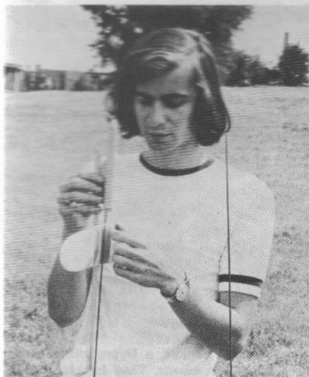
Max Yablonoitch preps his full-size "Jiskra" boost/glider which flew in the Sparrow B/G event. The Jiskra is a heavy model, but it showed excellent stability and a good glide during trimming tests. Unfortunately, the clip leads went up with the glider on the contest flight, putting it somewhat out of trim.
