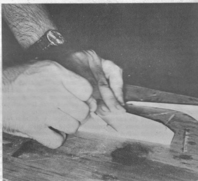
1. Mark the wing shape on a sheet of styrofoam, and use a sharp X-Acto knife to cut out the wing.
