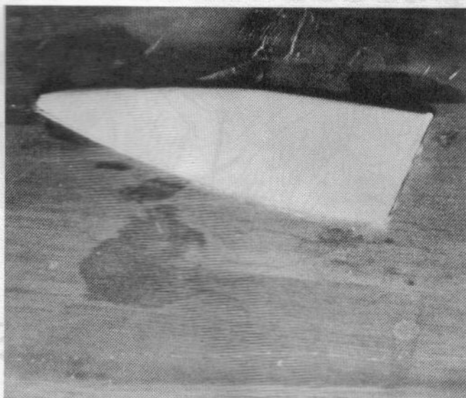
5. Cover the work board with wax paper, and lay the bottom of the wing flat on the waxed surface.
