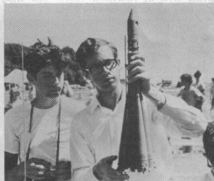
The Fleischer-Pearson Vostok, in 1:58.82 scale, turned in an excellent flight on an Estes D 13-3. This model showed good detailing on the strap-on weld patterns.
