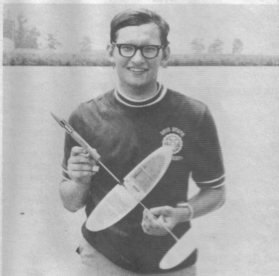
Chas Russell's 14" span cut-out wing B/G took first in Swift B/G with a 139.0 second duration. By removing sections of the wing and tissue covering, Chas reduced the weight of his B/G giving it a better glide.
