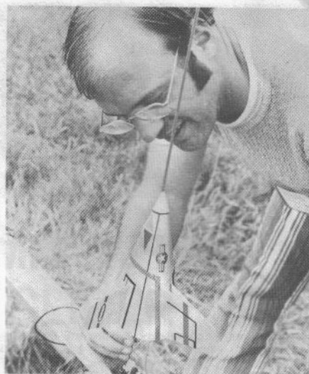
Larry Brown of Centuri Engineering preps the Centuri "Lifting Body," a unique gliding recovery model which made its first appearance at MMRR. This model generates lift for the gliding recovery by airflow over the body.
