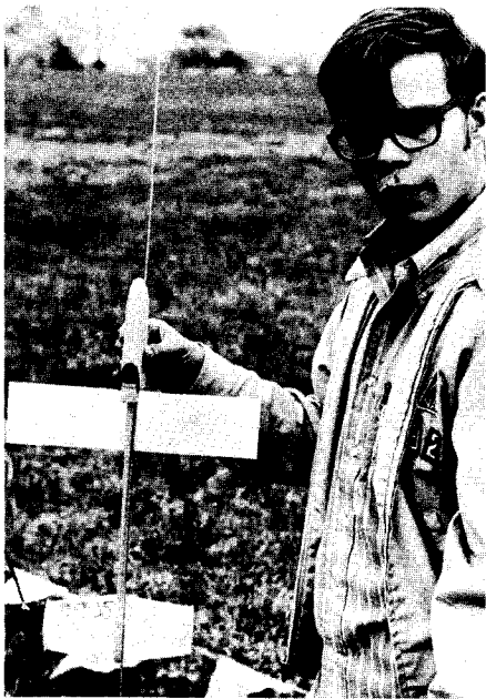
Carl Guernsey readies his "top and bottom" flop-wing for Condor B/G. The model used two E5-6's "because no E5-0's were available." Both ignited, and the boost was clean, but the model spiraled in for a DQ.
