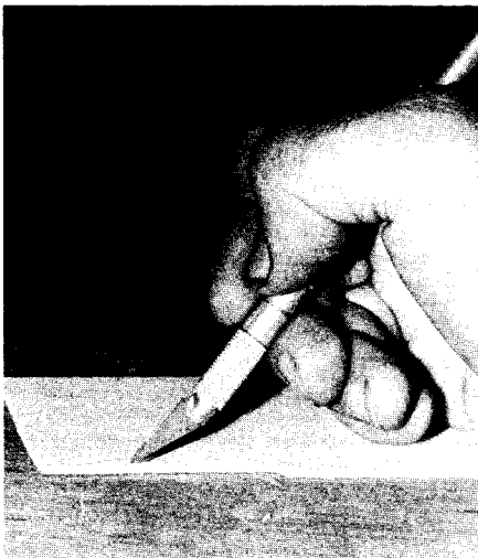
8. Cut a balsa strip to the correct thickness to serve as a center spar. Glue both sides of the spar. Insert the spar.
