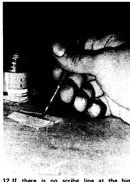
12. If there is no scribe line at the high point on the prototype, fill the scribe line with sanding sealer and sand smooth.
