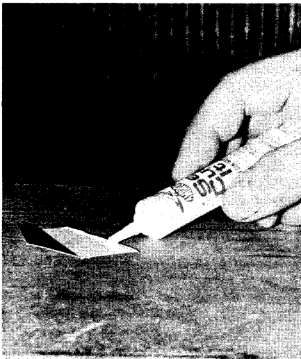
5. Apply a bead of non-water-base glue (such as Se-Cur-It or epoxy) to the inside edges of the fins, and spread it into a thin film.
