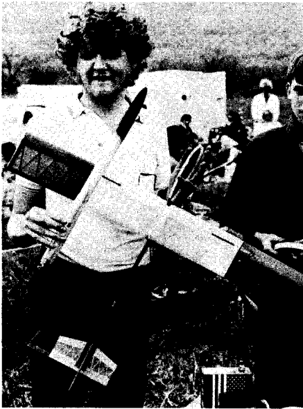
The only "standard configuration" B/G among the four top Condors was Bob Parks' radio-controlled flop-wing. Using single channel rudder only, Bob managed a duration of 119 seconds.
