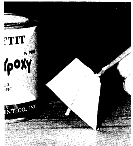
10. Use glue, wood filler, or Hobby epoxy "stuff" to fill in the tip edge of the fin. Do the same to the root edge.
