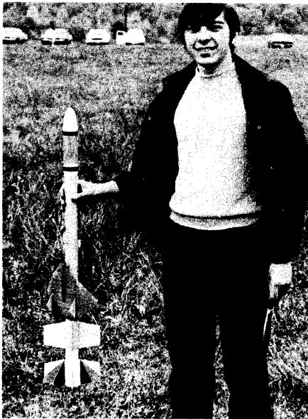
The Fox Team's parasite, which took fifth place overall, was a full size Manta on an Estes Omega booster. Powered by a D13-0 and E5-6, the glider managed a 99 second duration.
