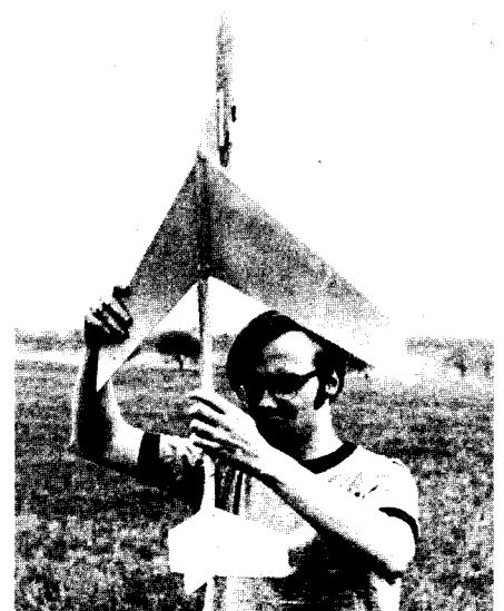
The "Super Thunder Bird," a double size Thunder Bird B/G, was built strongly enough that disintegration was no problem. But the glide trim was a little off, and the Kennedy-Gibbs team B/G spiraled in to a destructive impact.
