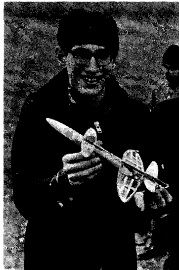
Contest Coordinator Doug List displays his unusual Sparrow B/G—a Bumble Bee parasite attached "backwards" to a normal sized model. This novel idea failed when the glider did not separate from the booster.
