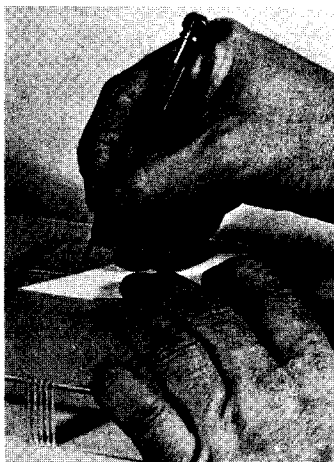
23. Four clear plastic fins are cut from the top of a plastic box or from Estes clear fin stock (CFS-40). The full size template at right should be used as a fin pattern. No additional nose weight is necessary if these fins are used.
