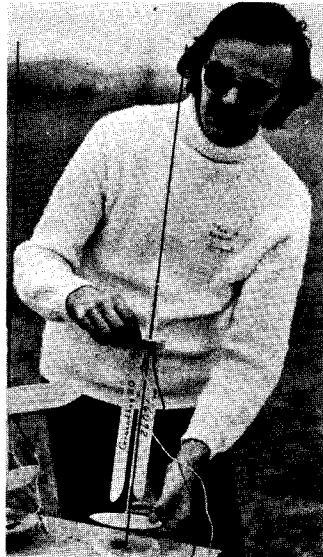
This unusual swing-wing entry was Jon Robbins' "Ground Hog" series—one in each size for the six B/G events. This one is the Sparrow, which boosted straight up but the right wing failed and the duration was only 12 seconds. Note the very high aspect ratio wings.
