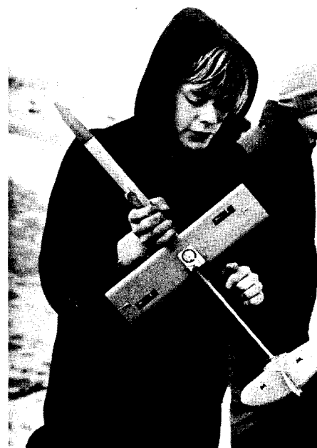
Steve Easley readies his "flop-wing" B/G for flight. The B/G used a Tatone dethermilizer timer to "pop-up" the tail and bring the glider down to avoid loss.
