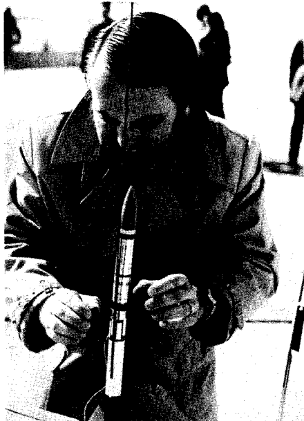
Dane Boles of Estes Industries demonstrates the new Estes "Transroc" model rocket transmitter. This version of the "Transroc" transmits a beacon signal to allow easy recovery of the model. The signal to allow recovery of the model. The launching rocket is an Estes Alpha III using the new plastic fin unit and nose cone.
