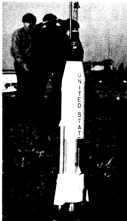
Anton Repa's beautiful model of Mercury Atlas 109-D flies with three 10 nt-sec engines. Small plastic fins are used to insure stability.
