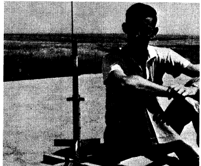
Del Hitch, NAR#3, poses with the first successful cluster-powered model rocket, TFB-3, at Green Mountain in June 1958. Unpainted test booster was made from paper towel core into which three engines would fit; upper stage was well-used Aerobee-Hi with cut-down fins.
