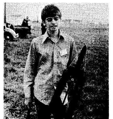
Mike Coxen of NARCAS displays his Condor B/G. This glider used swing wings folded back during boost (as above), and extended for glide. Unfortunately, this was one of the Condors not given an opportunity to fly.
