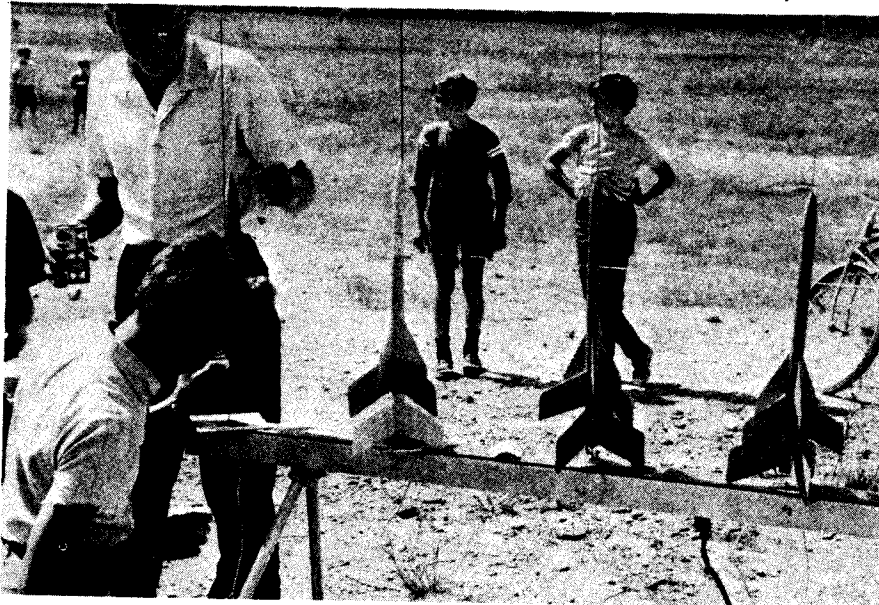
The Open Payloaders all looked the same — like Estes Farside Kits — powered by a D in each stage. But with 60 nt-sec total impulse and a light cloud cover it was too much for the trackers. Only a lucky few were tracked.
