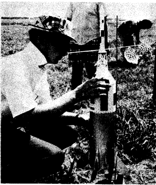
Scott Layne hooks up his 1/30th scale Little Joe II. The model, in 1/30 scale, was completely hand made with a balsa body tube and tower section fabricated from hardwood dowels. A perfect flight powered by an FSI F100 gave the model first in Junior Scale.
