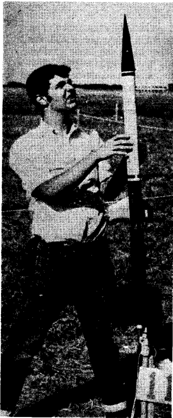
Alan Stolzenberg tries to stabilize his 5.54:1 WAC-Corporal. The three foot launch rod just wasn't long enough for his four foot tall model. Powered by an FSI F 100, the model weighed in at one pound. After an hour of work on the pad the WAC took off on a beautiful straight flight.
