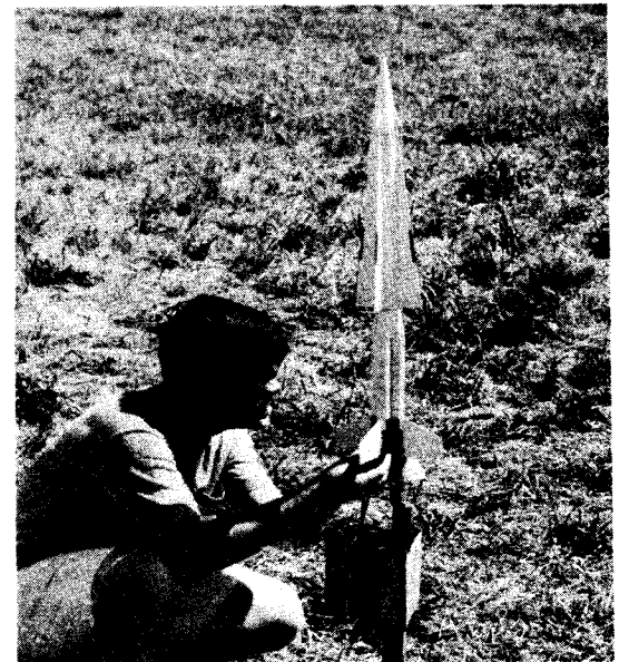
Gary Lindgren prepares a scale Nike-Hercules for a demonstration flight. Gary flew the model two-staged, with a ducting system to carry the booster engine ejection charge to the upper stage nozzle. His experiments have indicated that the system can be used over distances to 10 inches.
