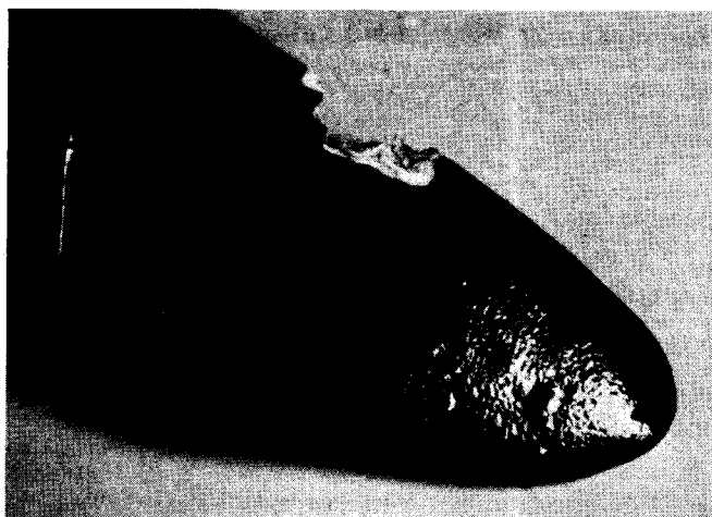
1. Since balsa is lighter than epoxy, try to reposition any small fragments of the fin and reshape it as much as possible.
