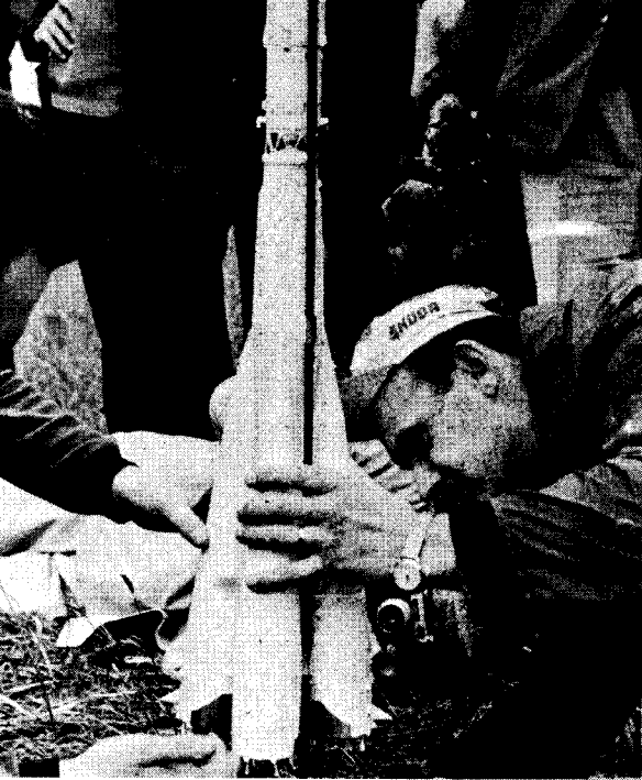
At left Jerabek of Czechoslovakia prepares the 1st place winning USSR "Vostok." Notice the detail, especially on the interstage adapter. Above, Jerabek's "Vostok" lifts-off on its prize winning flight. The model was powered by four 10 nt-sec Adast motors.
