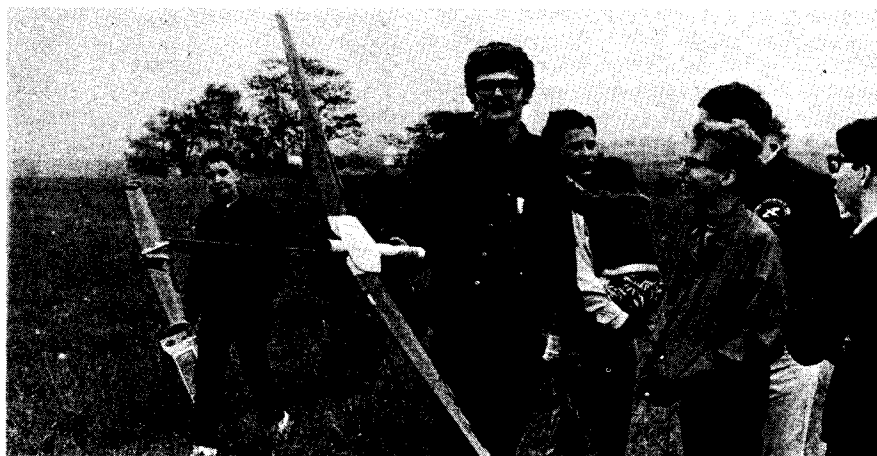
Jim Sparks explains the operation of his variable geometry B/G design. The wings fold back against the body during boost, and extend during glide. Unfortunately the T-tail caused the boom to snap during the boost phase of flight.
