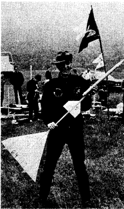
Bruce Blackistone (left) displays his "indestructible" B/G, the Disaster 17-B, just before its first — and last — F100 powered flight. All the parts of its shattered wing were recovered and reassembled (right) to evaluate the cause of the failure. The conclusion: even ¼" thick balsa can't stand up to F100 power.
