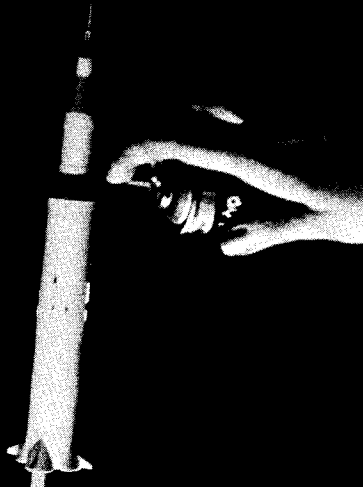
Glue the Apollo capsule to the front of the body. Press, do not cement, the escape tower into place. Now, spray the entire rocket with flat white enamel.
