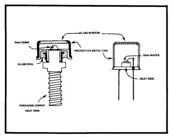
Fig. 4. Two common types of light emitting diodes. The one on the left is the type used in the report.
