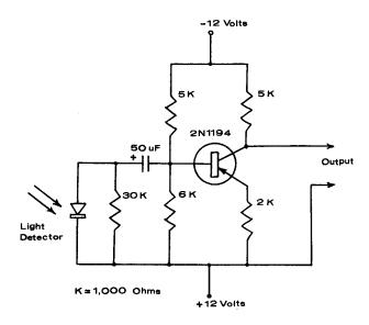
Fig. 9. The advanced experimenter will want to consider circuits such as this for improving performance of the light beam receiver.
