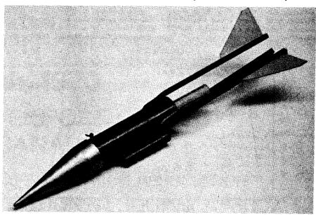
An original Carlisle Mark I, the world's first model rocket. Body is one inch diameter, stilts are balsa, fins are tag board. Nose cone is made from paper. The Mark I had parachute recovery. This model is destined for the Smithsonian Institution.
