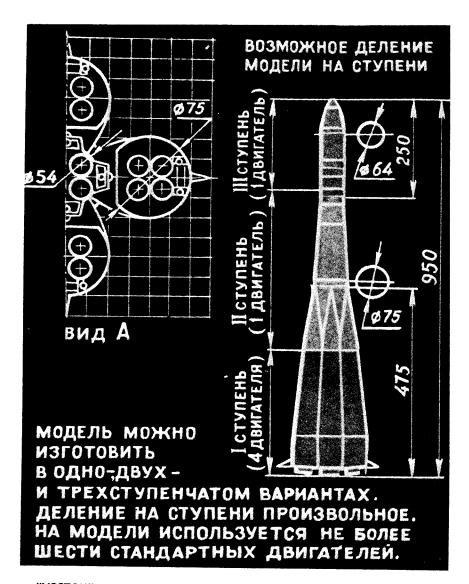
"VOSTOK" model drawing from Novosti. Model dimensions in millimeters are shown. Suggested divisions into stages (for a multistage model) are shown.
