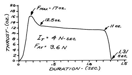
STATIC TEST DATA: Carlisle Type 4-4-1, hand-loaded by Orville H. Carlisle, April 1958. Tested September 13, 1962 on RDC Model 62A1 static test stand.
