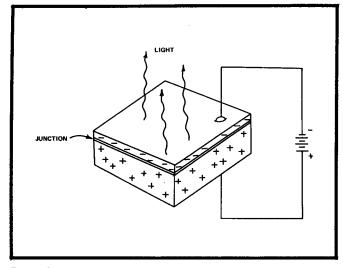
Fig. 5. Principle of light generation by a simple light emitting diode. Light is generated at the junction of positive and negative light emitting material when a small voltage is applied.
