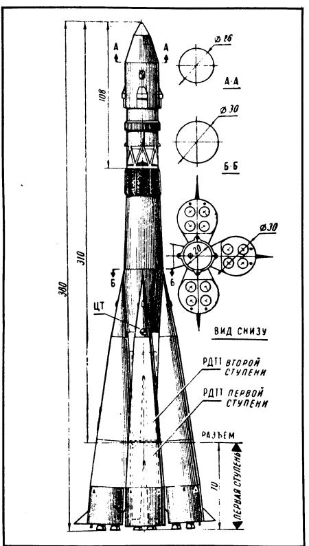
"VOSTOK" drawing, showing prototype dimensions in decimeters (ten decimeters equals one meter). This Russian drawing was supplied by Novosti Press Agency. The Russian inscriptions read (from top to bottom): Bottom View; Rocket Engine of the Second Stage; Rocket Engine of the First Stage; Connector; First Stage.
