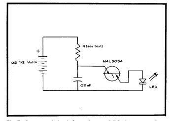
Fig. 7. A suggested circuit for an improved light beam transmitter. The M4L3054 is a four-layer diode.
