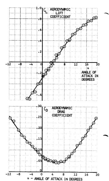
The Nighthawk's Lift, Drag, and Pitching Moment variations with angle-of-attack (a) have been plotted in coefficient forms (CL, CD, and  $C_{Mcg}$ ). In addition, the Lift-to-Drag Ratio ( $C_L/C_D$ ) and Aerodynamic Glide Factor ( $C_L^{3/2}/C_D$ ) graphs have been lined up with the Pitching Moment graph so that glide performance at the trim position can be more easily illustrated.
