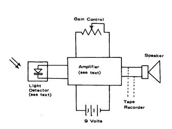
Fig. 8. As shown by this block diagram/circuit, the original receiver is quite simple. Not shown in the diagram is the lens or parabolic reflector used to collect light from the light beam transmitter.
