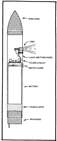
Fig. 2. Payload III showing the light emitting diode pointing from the side. The lens was used only on Payload I and is included here to show its location.
