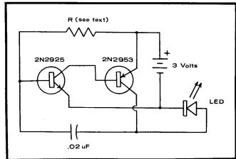
Fig. 6. Schematic of the original circuit used in Payloads I, II, and III. Resistor "R" controls the frequency of the circuit as explained in Appendix 3.
