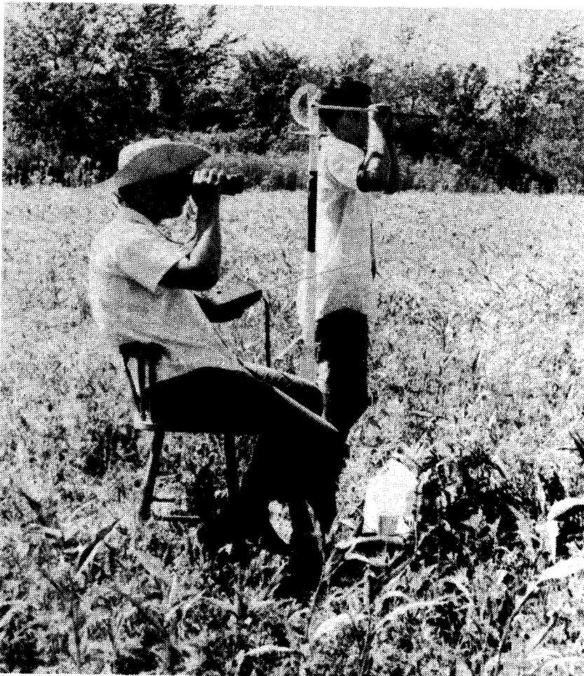
Tracking west is Go! As Mark Maselli handles communication with data reduction, Jon Bonine (R) mans the Ball-Hagedorn rear-pivot theodolite.
