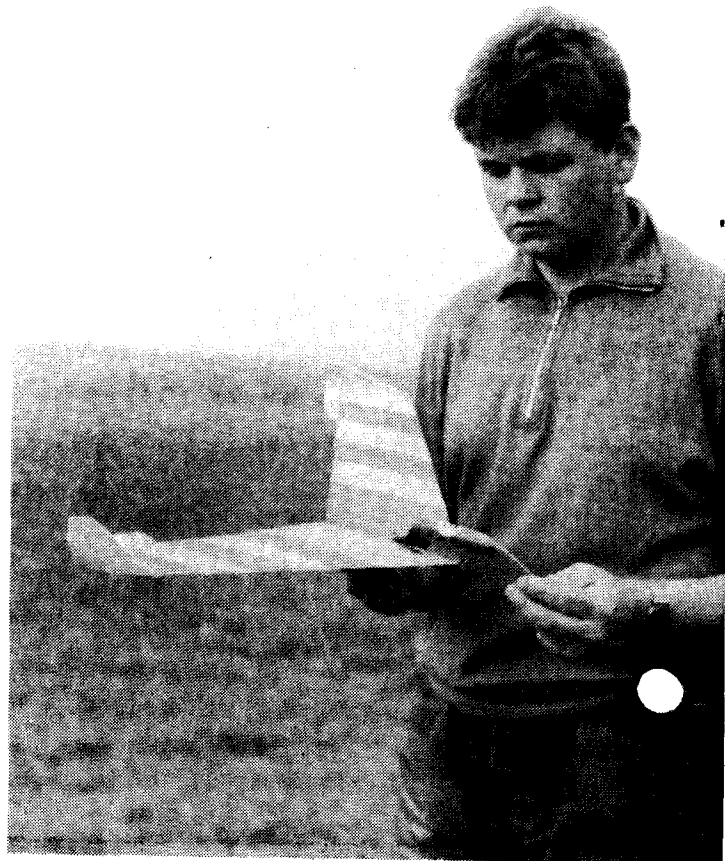
Premysl Kynel (below) of Radotin displays a destructed scale Aerobee-Hi. The Class II scale model had been flown with a 5 Newton-second engine in each stage.
