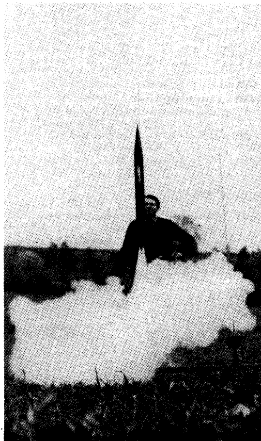
Jaroslav Divis of Praha prepares his scale Class III Sergeant. This model employs a cluster of four 10 Newton-second engines, as can be seen from the second photograph. A 50-inch parachute was used on the model, and a six-second delay was employed in the engines.
