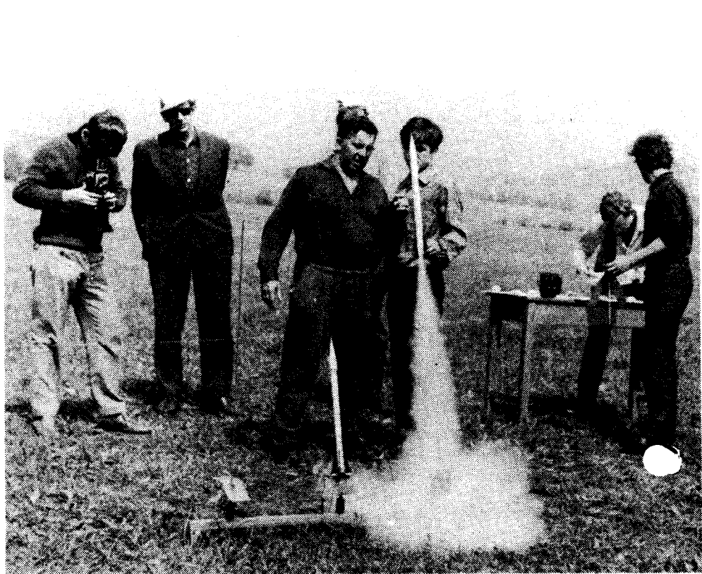
Liftoff of Frank Brehovy's scale ASP powered by a single 10 Newton-second engine.
