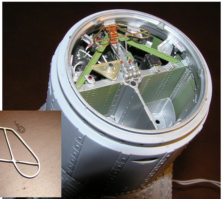
Figure 28. The left image shows the kit part with new interior wall and rivets all over the place. I estimated that about 1,000 rivets were added to this piece along. The second image shows the cruciform structure upon which the components are attached. The parachute compartment is to the right, and is empty after recovery because the chutes have deployed. The right image shows a sample of some of the equipment boxes. Much of the equipment opposite the parachute compartment are made up, as detailed information about what's in here doesn't seem readily available. Good photos of the top portion did help in at least trying to make this section look mostly accurate. It was fun to create the equipment boxes and hook them all up to wiring harnesses.
